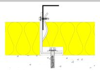
The insulation will have to be cut away to allow the leg of the rails to be fitted but will not affect the fixing of the rail to the bracket.
