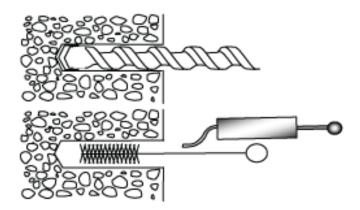
When fixing FastFrame brackets into concrete, a pull out test must be performed to verify the strength of the masonry. All drill holes should be thoroughly cleaned out and free from dust and grit before fixings are inserted.
