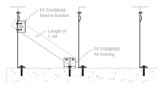
All stand offs greater than 300mm should be cross braced as per the detail shown here. This needs to be on the top and bottom bracket of one rail every 3m going across the facade. We do not advise that you
