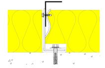
The insulation will have to be cut away to allow the leg of the rails to be fitted and the rail to bracket fixing is inder the surface of the insulation making it very hard to fit.
