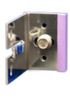
When fixing FastFrame brackets into concrete, ensure the fixings are placed in the larger elongated holes with the collar of the frame anchor plug on the face of the bracket.
