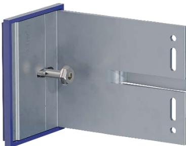
When anchoring F1 consoles on steel or wooden surfaces, make sure that the number of anchoring screws equals the number of fixing holes per bracket. The anchoring must be done in all 6.5mm slots of the console.
